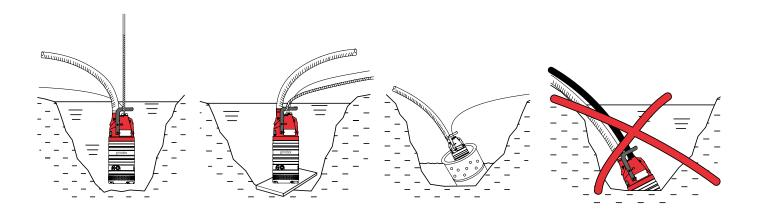
Arrange the pump so it doesn't burrow itself into sand or clay. This is a common problem at construction sites. It can be avoided quite simple by placing the pump on a bed of coarse gravel or a plank. The pump can also be hung freely by a rope or chain, or put into a cut-down and perforated oil drum.
